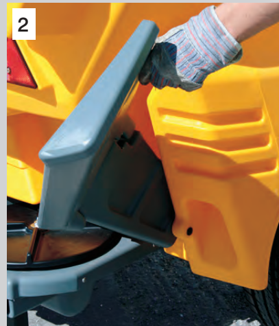
2 Lower the first side deflector into position.
